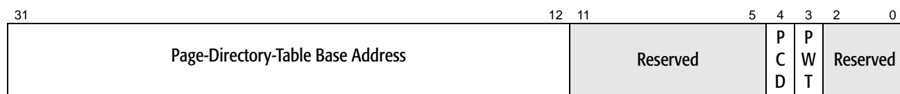
Figure 3-4. Control Register 3 (CR3)—Legacy-Mode Non-PAE Paging
